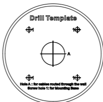
Figure 2-9 Drill Template of the Junction Box
